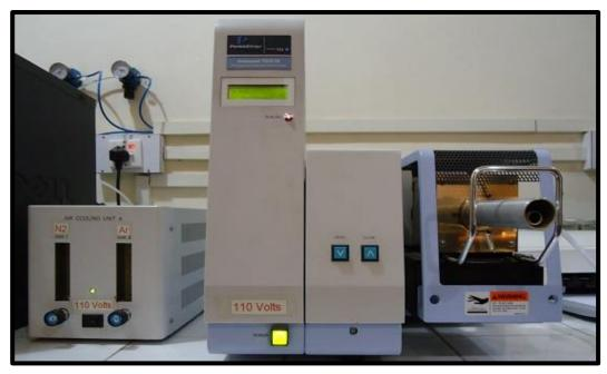
Figure 2.5: Thermogravimetric/differential thermal analyzer
