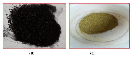
Figure 3.3: (A) Flowchart for the preparation of Ba<sub>0.6</sub>K<sub>0.4</sub>BiO<sub>3</sub> (B) Ba<sub>0.6</sub>K<sub>0.4</sub>BiO<sub>3</sub> powder precursor at 350° C/2h. (C) Ba<sub>0.6</sub>K<sub>0.4</sub>BiO<sub>3</sub> perovskite at 720° C/12h.
