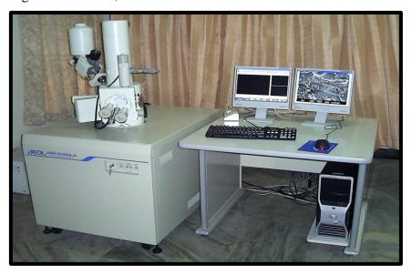
Figure 2.9: Field emission gun-scanning electrone microscope.
