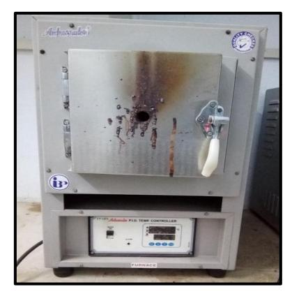
Figure 2.1: Muffle Furnace
