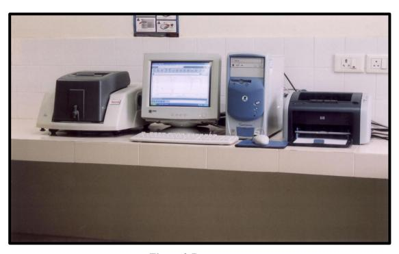
Figure 2.7: FT-IR Spectrometer
