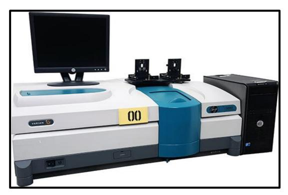
Figure 2.8: UV-Vis Spectrophotometer
