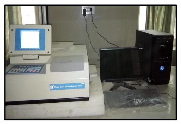
Figure 2.3: Double beam spectrophotometer.
