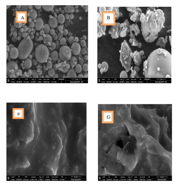
Figure 6.3: SEM micrographs (A) pure FA (B) MFA-40 (C, D) *N*-(3-(trimethoxy silyl)propyl)-*N*-(propyl-3-sulfonate) ammonium hydrosulfate/MFA and magnified image of Catalyst
