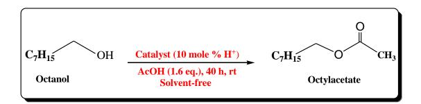
Scheme 1.52: IL@SBA-15-Pr–SO<sub>3</sub>H catalyzed esterification of 1-octanol with acetic acid
