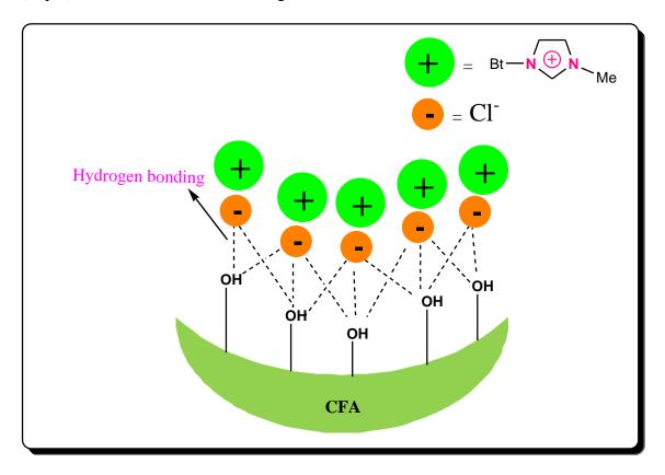
Scheme 3.5: The proposed structure of [bmim]Cl/CFA catalyst
