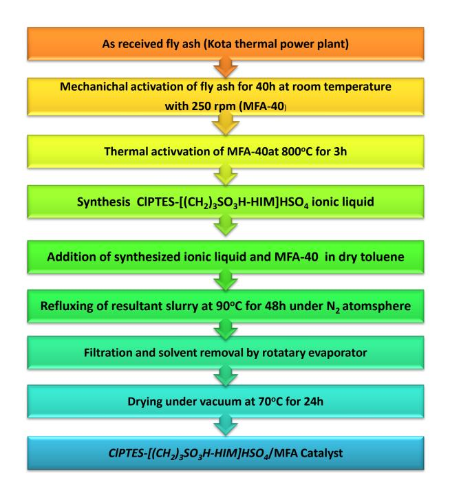
Scheme 5.2 : Steps for Synthesis of CIPTES-[(CH<sub>2</sub>)<sub>3</sub>SO<sub>3</sub>H-HIM]HSO<sub>4</sub>/MFA
