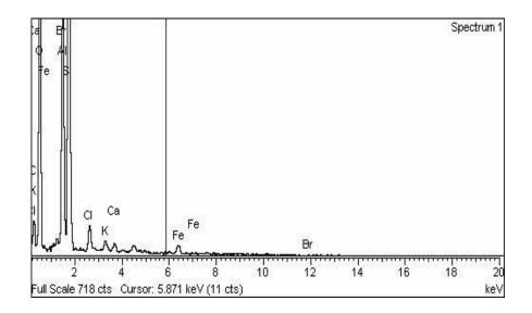
Figure 3.6: EDX spectrum of [bmim]Cl/CFA
