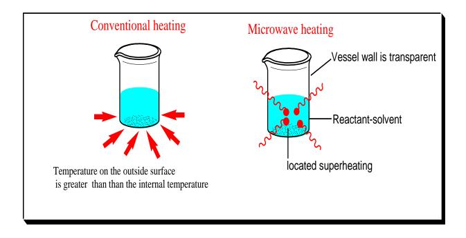
Figure 1.3 Difference between conventional and microwave heating
