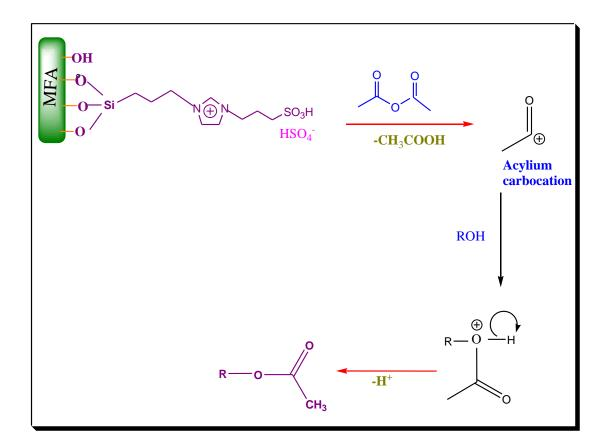
Scheme 5.5: Proposed mechanism of acylation of aromatic alcohol by acetyl
