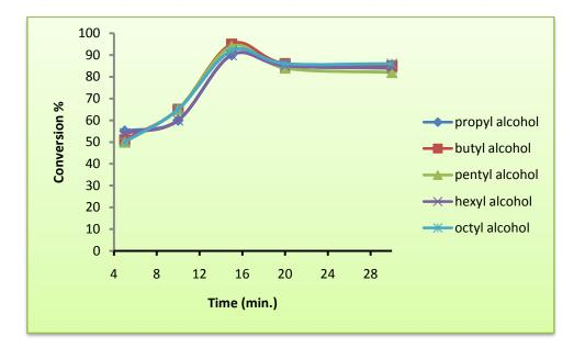
Figure 3.8: Variation of conversion% of alcohols over catalyst with time.
