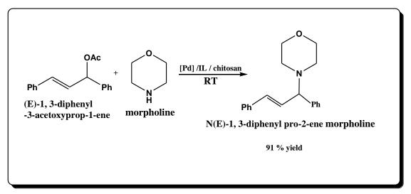
Scheme 1.48: Allylic substitution between morpholine and (E)-1, 3-diphenyl-3acetoxyprop-1-ene using Pd/IL/Chitosan
