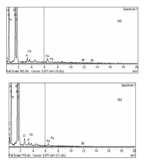
Figure 2.10: EDX spectrum of (a) MFA-40 (b) TMICl/MFA
