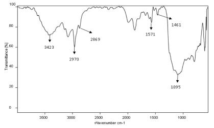
Figure 2 FTIR spectra of [bmim]Cl/CFA
