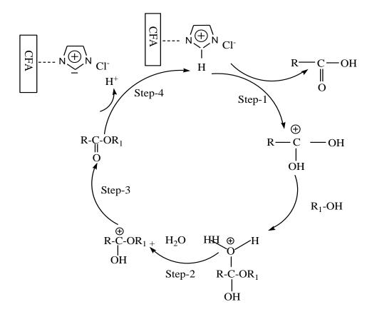
Scheme 3.6: Proposed mechanistic pathway of microwave-assisted esterification of propanoic acid with aliphatic alcohol over [bmim]Cl/CFA catalyst
