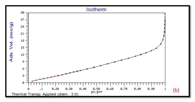
Figure 2.6: (a) Pore distribution curve of MFA-40, (b) B.E.T. adsorption isotherm of MFA-40
