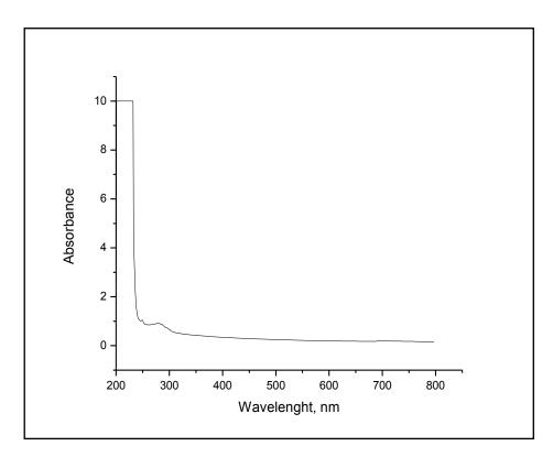
Figure 4.6 : UV-VIS spectrum for purity of [bmim]PF<sub>6</sub>
