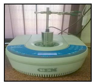
Figure 2.1: CEM Focussed Microwave <sup>TM</sup> Synthesis System (Discover Model)
