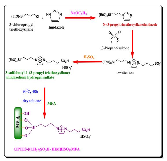
Scheme 5.1: The synthesis route of CIPTES-[(CH<sub>2</sub>)<sub>3</sub>SO<sub>3</sub>HHIM] HSO<sub>4</sub>
