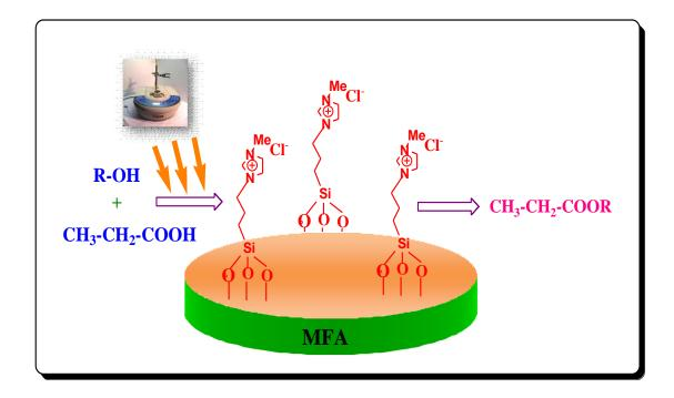
Esterification reaction over fly ash supported 1-methyl-3-[triethoxysilyl propyl]imidazolium chloride
