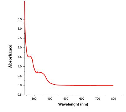
Figure 3.4: Uv-Visible spectra of [bmim]Cl/CFA
