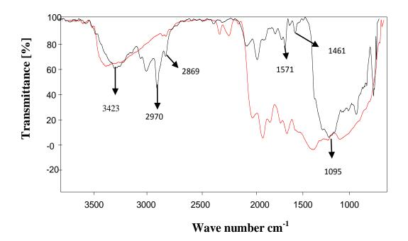
Figure 3.3. FTIR spectra of (i)CFA and (ii) [bmim]Cl/CFA
