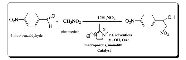
Scheme 1.49: Continuous-flow solvent less Henry reaction catalyzed by basic-SILPs.
