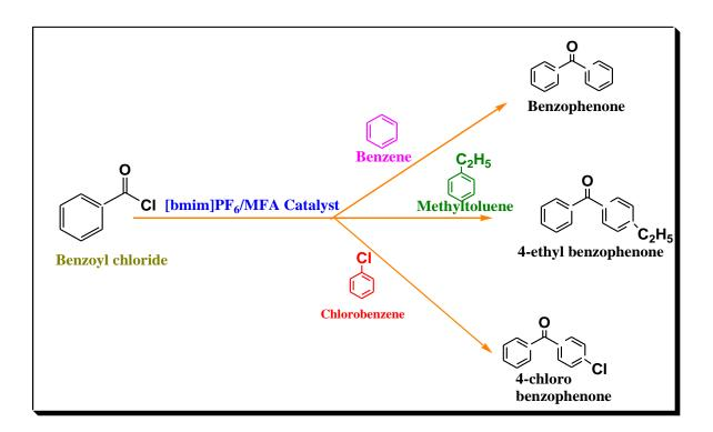
Scheme 4.3: Simplified reaction pathway of benzoylation of aromatic substates by benzoyl chloride over [bmim]PF<sub>6</sub>/MFA catalyst to give corresponding benzophenone and its substituents.
