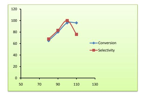
Figure 4.8: Variation of conversion and selectivity (%) of methyltoluene over [bmim]PF<sub>6</sub>/MFA with temperature.
