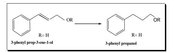
Scheme 1.47: Hydrogenation of a variety of olefins Pd-SH-SILC
