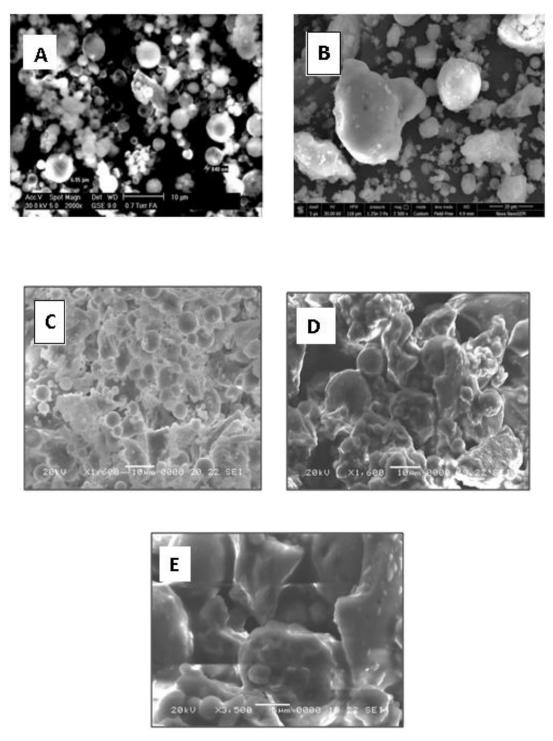
Figure 2.9 : SEM micrographs (A) pure FA (B) TMICL/FA (C) MFA-40 (D, E) TMICI/MFA and magnified image of TMICI/MFA
