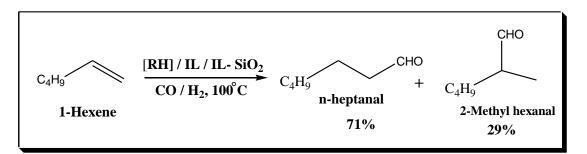
Scheme 1.44: [Rh/IL/IL-SiO<sub>2</sub>]catalyzed hydroformylation of 1-hexene
