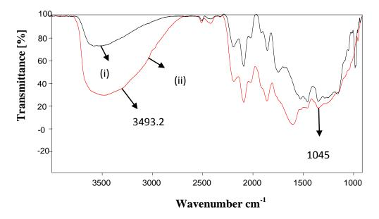
Figure 3.2. FTIR spectra of (i) FA (ii) CFA
