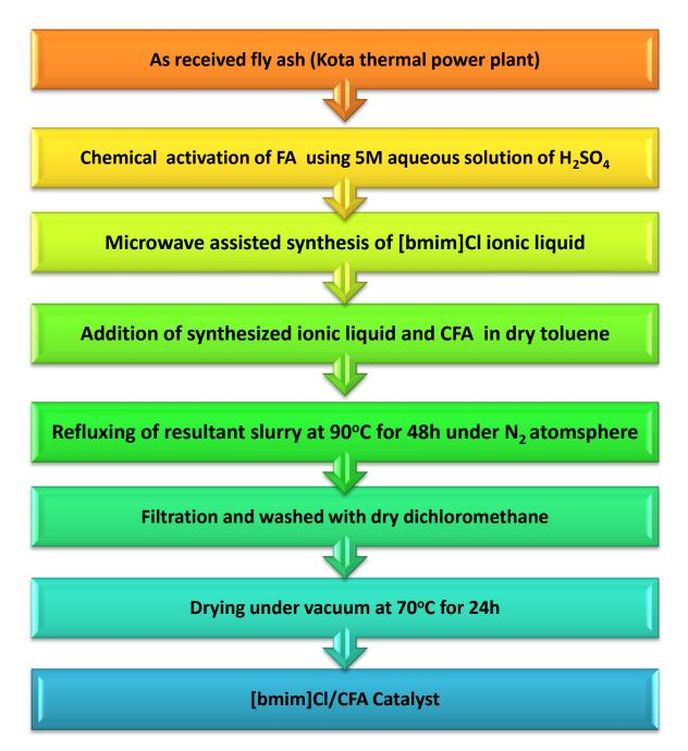
Scheme 3.3: Steps for synthesis of [bmim]Cl/CFA catalyst
