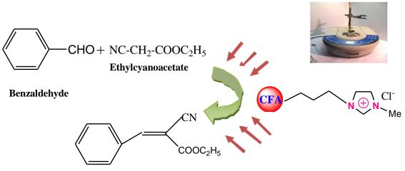
ethyl 2-cyano-3-phenylacrylate Scheme 1 The Knoevenagel condensation of benzaldehyde and ethyl cyanoacetate
