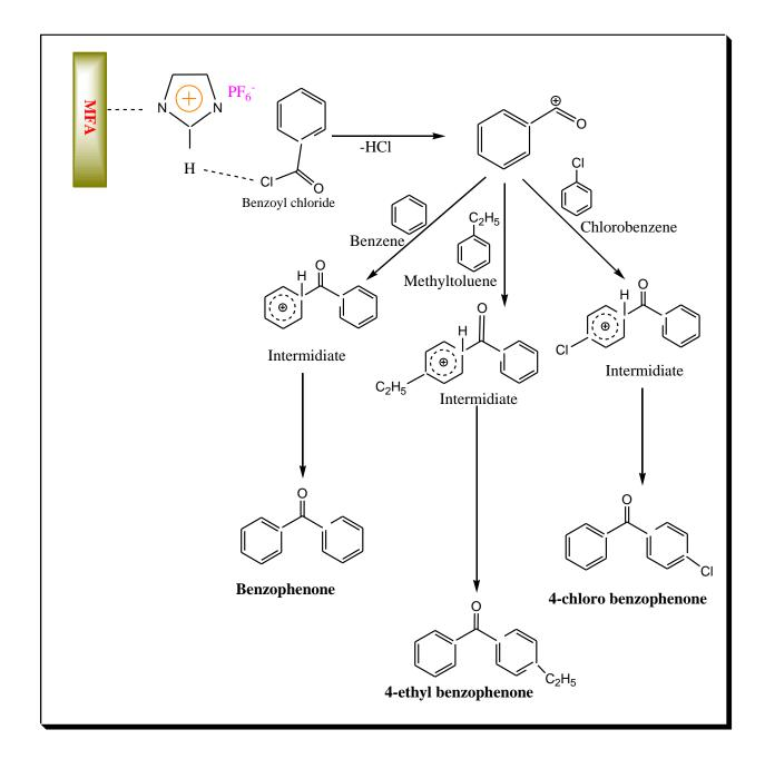
Scheme 4.4 : Proposed mechanism of benzoylation of aromatic substrates using benzoyl chloride over [bmim]PF<sub>6</sub>/MFA
