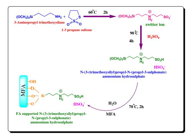
Scheme 6.2: The synthesis route of N-(-3-(trimethoxy silyl) propyl-N-(propyl-3sulfonate) ammonium hydrosulphate functionalized FA.
