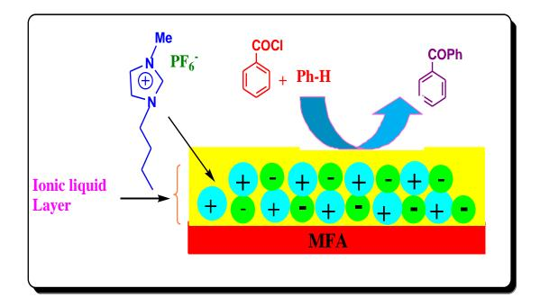
Benzoylation reaction over fly ash supported 1-butyl-3-methylimidazolium hexafluorophosphate catalyst
