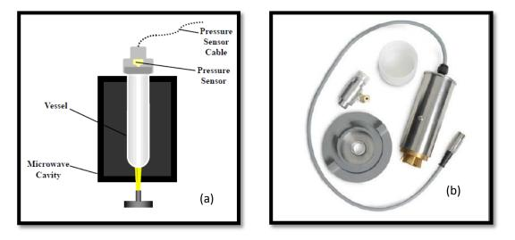
Figure 2.2: (a) Infrared temperature sensor and (b) Intellivent pressure sensor assembly
