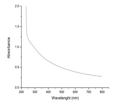
Figure 5.2 : UV-VIS spectrum of purity of ionic liquid
