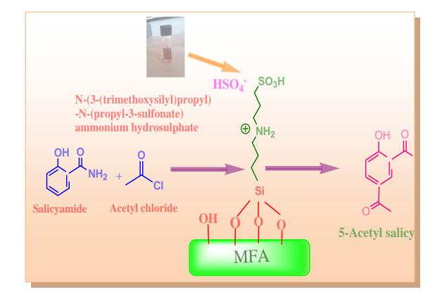
Freidel Craft Acylation reaction of Salicylamide over *N*-(3-(trimethoxysilyl)propyl)-*N*-(propyl-3-sulfonate) ammonium hydrosulphate/MFA
