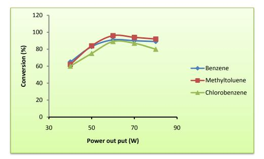
Figure 4.14: Variation of conversion % of benzene, methyltoluene, chloro benzene over [bmim]PF<sub>6</sub>/MFA with power output.
