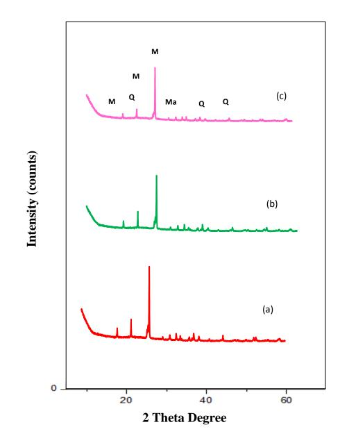
Figure 2.7 : X-ray diffraction patterns of (a) Pure FA, (b) MFA-40 (c) TMICI/MFA
