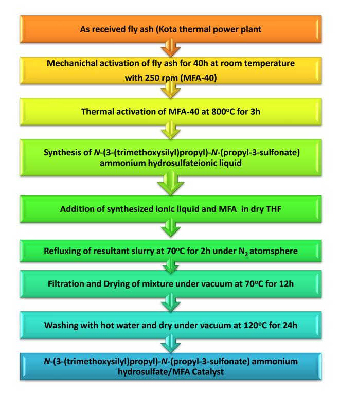
Scheme6.3: Synthesis of FA supported ionic liquid catalyst (*N*-((trimethoxysilyl)
