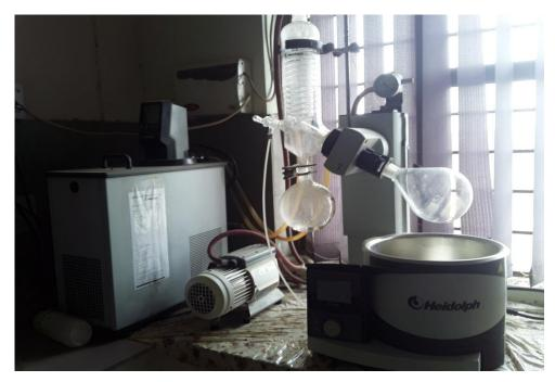
Figure 2.3 : Rotary evaporator (Heidolph G3, Germany)
