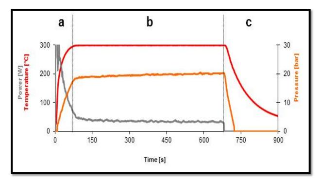
Figure 2.5 : Temperature and power profile of microwave experiment
