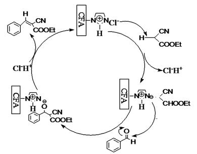
Scheme 2 Proposed mechanistic pathway of microwave-assisted condensation of benzaldehyde and ethyl cyanoacetate reaction over [bmim]Cl/CFA catalyst
