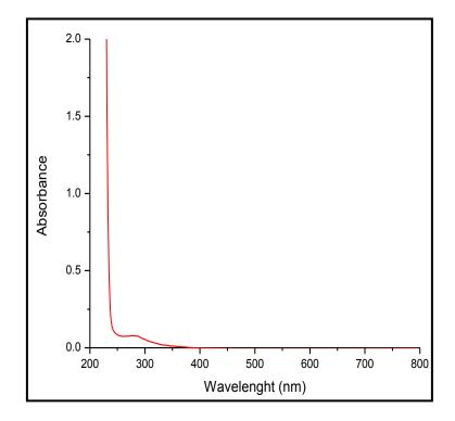
Figure 6.2 : UV-VIS spectrum for purity of *N*-(3-(trimethoxysilyl)propyl)-*N*-(propyl-3-sulfonate) ammonium hydrosulfate
