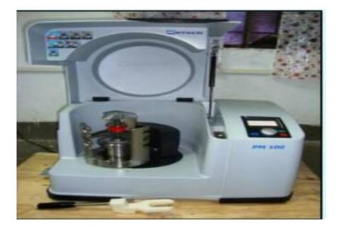
Figure 2.4: RETSCH Planetary Ball Mill
