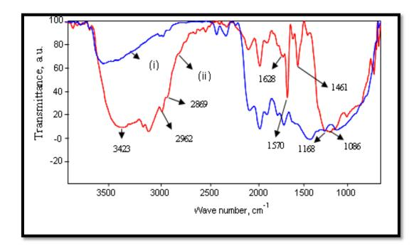
Figure 2.9: FTIR spectra of (i) MFA-40(ii) TMICl/MFA
