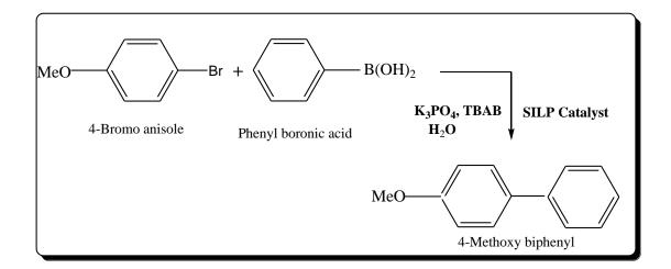
Scheme 1.43: [tpim] [Cl]/ MFI zeolite catalyzed Suzuki coupling reaction between aryl bromides and arylboronic acids.
