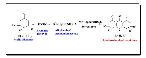
Scheme 1.54: Synthesis of Decahydroacridines over MNP-[pmim]HSO<sub>4</sub> catalyst
