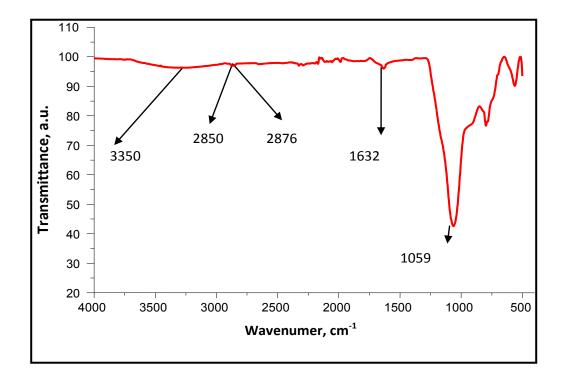
Figure 6.1: FT-IR spectra of *N*-(3-(trimethoxysilyl)propyl)-*N*-(propyl-3sulfonate) ammonium hydrosulfate/MFA catalyst
