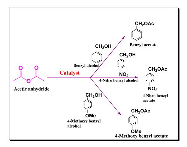
Scheme 5.3: Simplified reaction pathway of acylation of aromatic alcohol by acetic anhydride over CIPTES-[(CH<sub>2</sub>)<sub>3</sub>SO<sub>3</sub>HHIM] HSO<sub>4</sub>/MFA.
