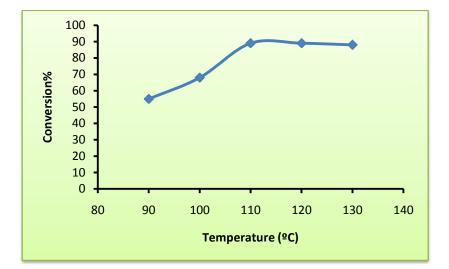
Figure 2.14: Variation of conversion (%) of propanoic acid over TMICl /MFA catalyst with temperature.
