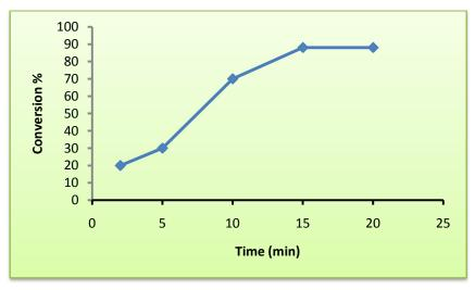
Figure 2.15: Variation of conversion (%) of propanoic acid over TMICl/ MFA catalyst with reaction time
