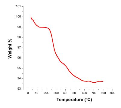
Figure 3.7. TGA pattern of [bmim]Cl/CFA
