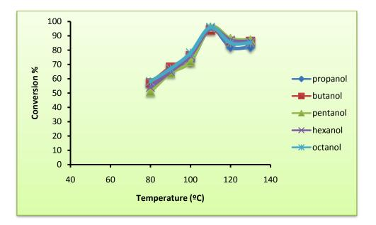
**Figure 3.7: Variation of conversion% of alcohol over catalyst with temperature.** Reaction conditions under microwave irradiation: Power = 100W; Pmax = ON; time = 15 min, molar ratio(aliphatic alcohol/butyric acid)=1:2, substrate/catalystratio=5:1
