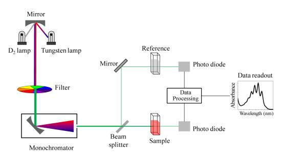
Figure 2.2: Schematic of a double beam UV-Vis spectrophotometer.
