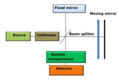
Figure 2.1: Block diagram of an FT-IR spectrometer [5].
