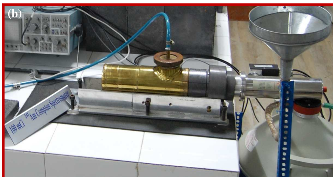
Fig. 2.6: (a) Layout of 100 mCi ^{241}\text{Am} Compton spectrometer. (1)- ^{241}\text{Am} -isotope; (2)-sample position; (3)-Ge crystal; (4)-HPGe detector capsule; (5)-lead shielding around source and detector; (6)- port for evacuation connected to rotary oil pump; (7)-scattering chamber made of brass; and (8)-mylar foil (25 \mu\text{m} ) to evacuate scattering chamber. (b) Laboratory view of the spectrometer at M.L. Sukhadia University, Udaipur.
